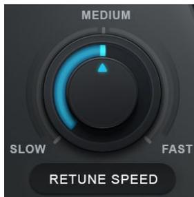
Set the Retune Speed to determine how quickly Auto-Tune Access tunes your audio to the target pitches.
