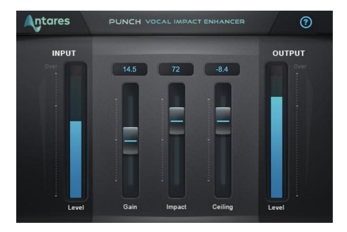
**Punch** is a dynamics processor that gives your vocals more dynamic impact. It provides a combination of compression, gain, limiting, and overload protection with an interface designed for speed and simplicity.
